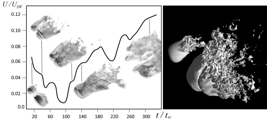
FIGURE 3. Drift rate fluctuations during the temporal evolution of two cloud structure.
