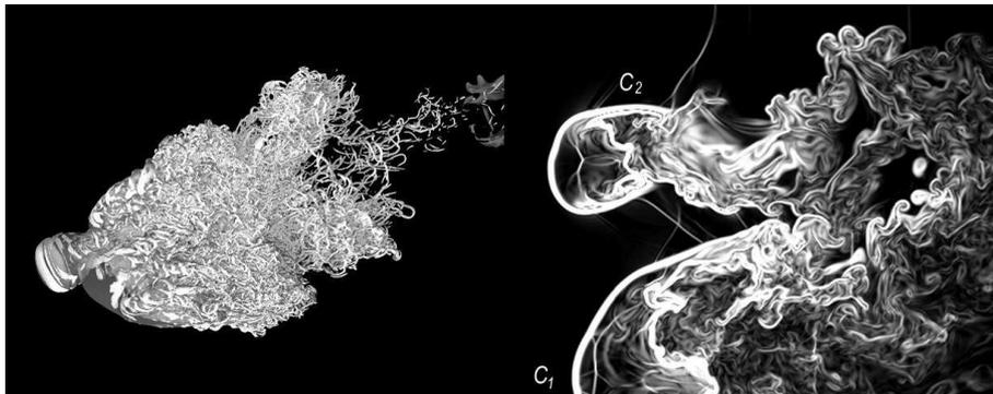
FIGURE 2. Vortex Q-criterion ( $Q = 100 \text{ s}^{-1}$ ) distribution and zoom-in of numerical schlieren for instantaneous density-gradient field at stage  $t = 75t_{sc}$ .
